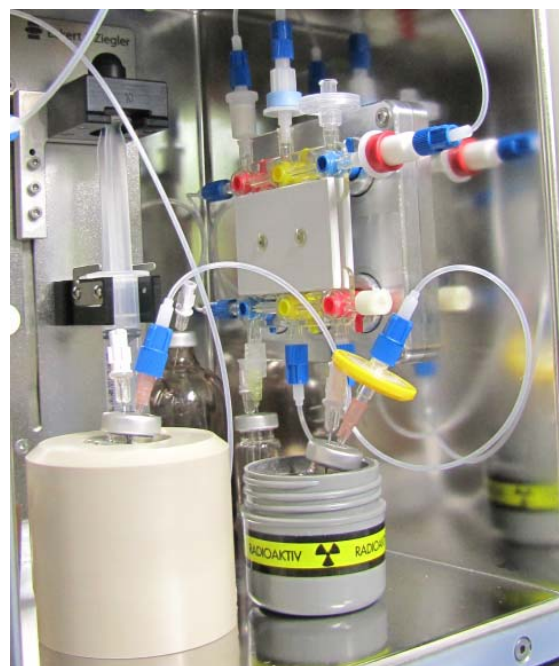
Inside shielding: cassette with syringe, heater and product vial
